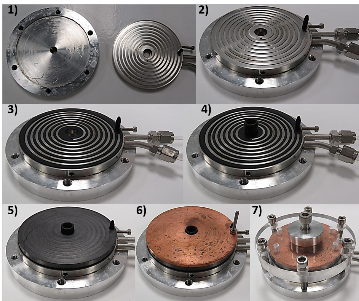
Figure 5 – Steps illustrating the construction of the Ammonite reactors.
