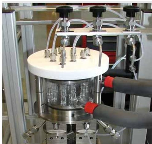
Oscillatory flow is useful wherever immiscible phases need to be mixed or slurries need to be managed and as such has found application in fine chemicals, waste water treatment and biofuels production, amongst other areas.
