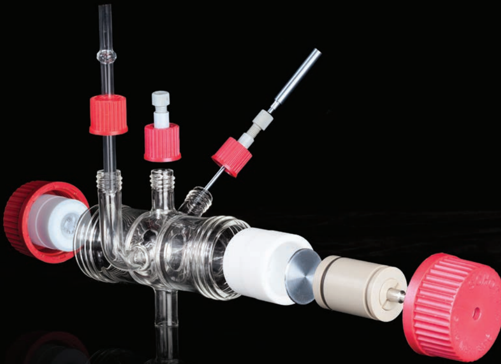
Exploded View. Conventional Three-Electrode Cell - Glass Construction
