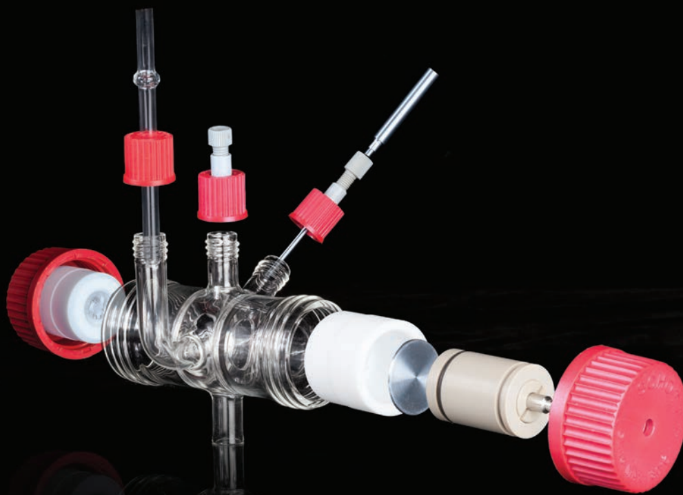
Exploded View. Conventional Three-Electrode Cell - Glass Construction
